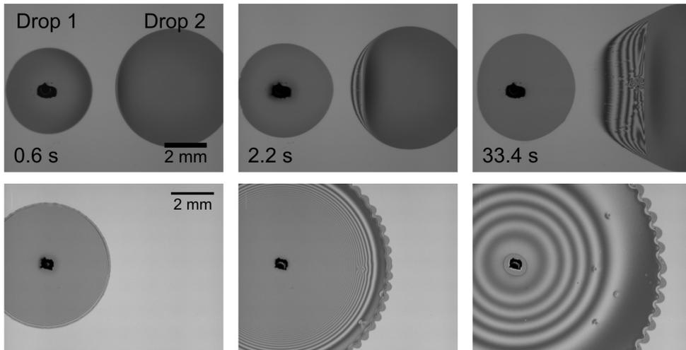
FIG. 1: **Top:** Interaction of left drop (volatile liquid, lower surface tension) with right drop (non-volatile liquid, higher surface tension). **Bottom:** Single droplet of a mixture of C9 and C16 alkanes spreading.
