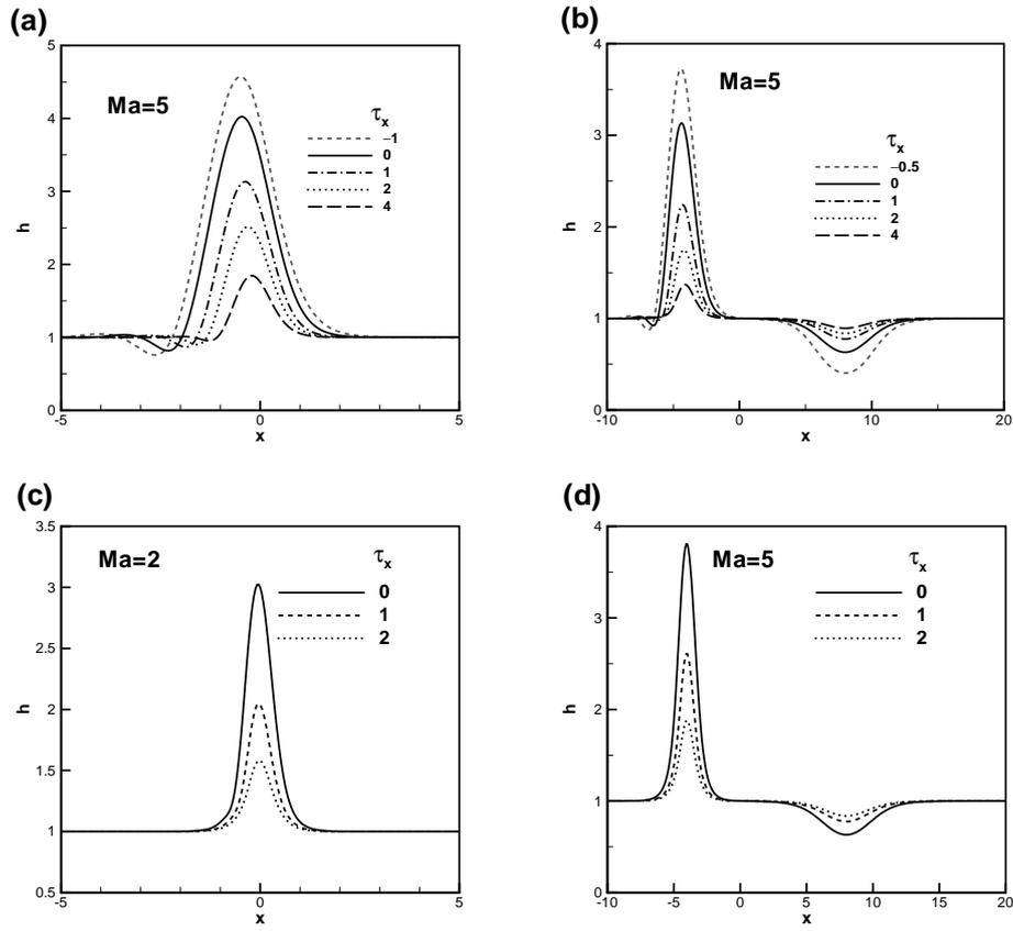
FIG. 1: Effect of interfacial shear on the film profiles for the steady solutions at  $Bi = 0$ . (a),(c) for semi-infinite heater with  $l = 20L$  and the wavelength  $\lambda = l/L$ , (b),(d) for finite length heater with the wavelength  $\lambda = 40$ .  $Bo = 10$  for (a) and (b), and  $Bo = 1000$  for (c) and (d).
