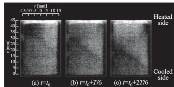
Fig. 2 Temperature fields measured by IR camera.
