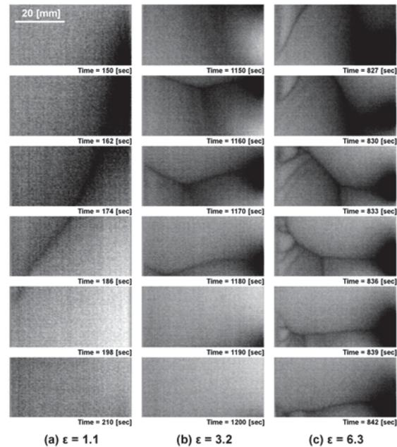
Fig.2. Time series of temperature deviation on the liquid bridge surface of  $1/6$  region in azimuthal direction evaluated by IR images in the case of  $\Gamma = 2.0$ ;  $(Ma, \epsilon) =$  (a)  $(4.2 \times 10^4, 1.1)$ , (b)  $(8.5 \times 10^4, 3.2)$  and (c)  $(1.5 \times 10^5, 6.3)$ .
