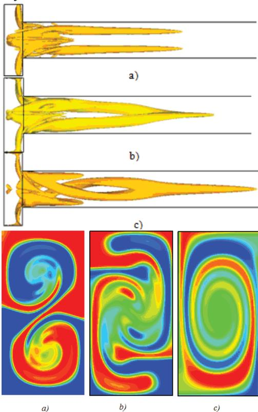
Flow vortex structure and contours of mass fraction of dye in the outlet of microchannel at various value of the slip length  $b$ .  $Re = 186$ . a)  $b = 0$ ; b)  $b = 10\ \mu\text{m}$ ; c)  $b = 30\ \mu\text{m}$ .
