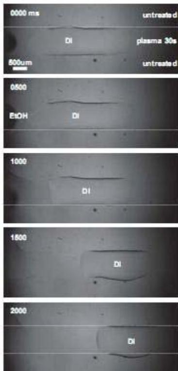
Fig. 1: Droplet actuation on a hydrophilic stripe.
