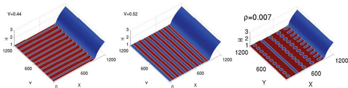
FIG. 1: Examples of patterns generated by monolayer transfer: Stripes oriented perpendicular (left) and parallel (center) to the contact line are observed for low and high pull velocities, respectively. Using prepatterned substrates, more complex structures can be realized (right).
