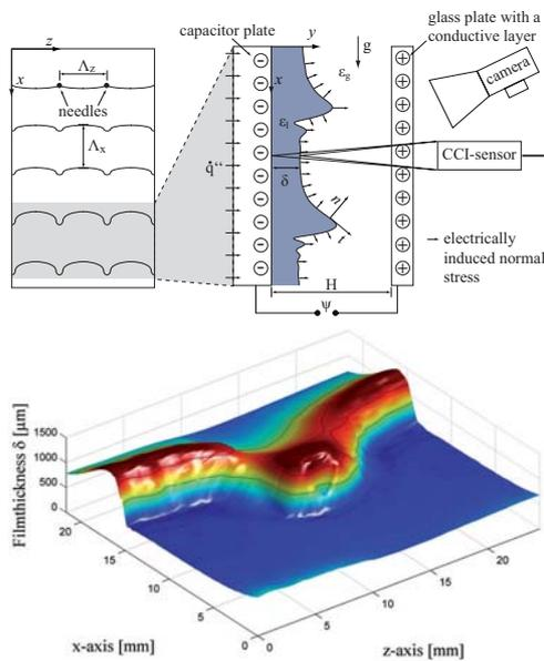
FIG. 1: Top: schematic drawing of the experimental setup: front view (left) and side view (right); Bottom: reconstructed three-dimensional plot from the surface waves with contours shown for  $900\mu\text{m}$ ,  $1200\mu\text{m}$ .
