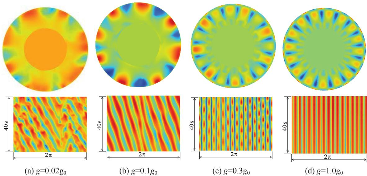
Fig. 1 Flow pattern transition process at  $\Delta T=10\text{K}$ . Upper plot: snapshots of surface temperature fluctuation; Down plot: space-time diagram of surface temperature distribution at a given radius
