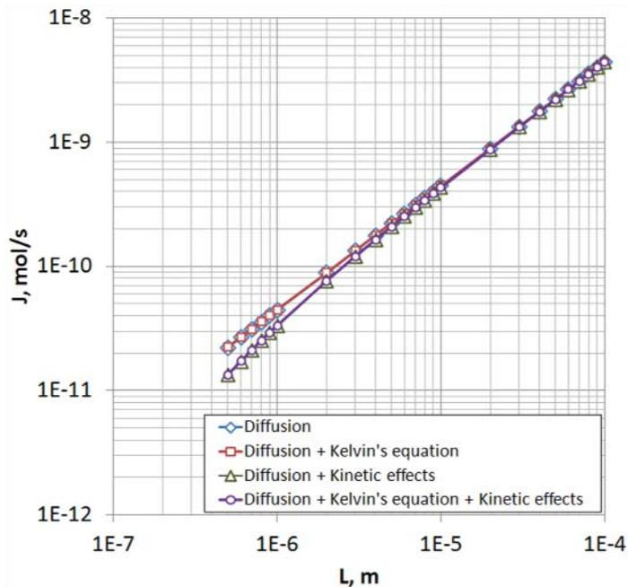
Fig. 1. Example of computer simulated dependence of evaporation rate,  $J$ , of a droplet on the contact line radius,  $L$ , in the case when contact angle is 90 deg. Parameters used: pure water droplet, copper substrate, air atmosphere, ambient temperature is 20°C, and relative air humidity is 70%.
