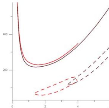
FIG. 1: Neutral curves for parametric Marangoni instability  $M(k)$  for  $\omega = 0.5$  (red color) and  $\omega = 2$  (brown color).  $P = 7$ ,  $B = 0.2$ ,  $L = 0.01$ ,  $N = 0.1$ ,  $\delta = 1$ . Solid (dashed) lines correspond to synchronous (subharmonic) mode.
