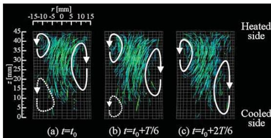
Fig. 1 Flow fields measured by 3-D PTV.
