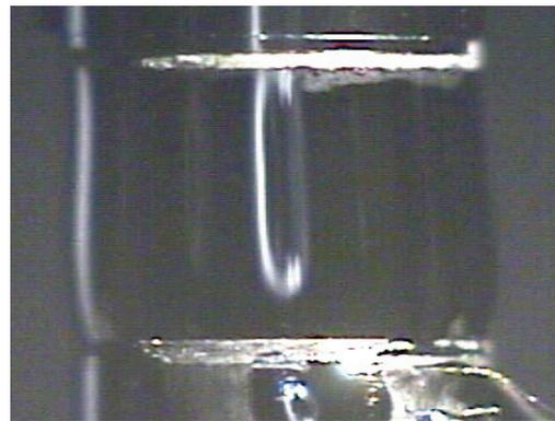
Fig.2 Liquid bridge of molten tin (Pr=0.009) with 6 mm diameter and 4.2 mm length
