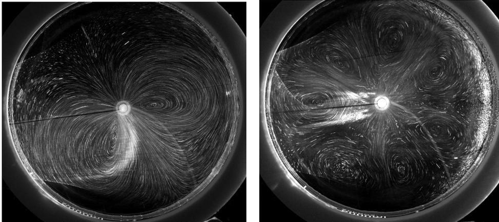
FIG. 1: The surface flow structure under  $Ma = 2 \cdot 10^6$  and surfactant surface density  $\Gamma/\Gamma_e=0.35$  (left picture) and 0.3 (right picture).  $\Gamma_e$  - surface density of monolayer.
