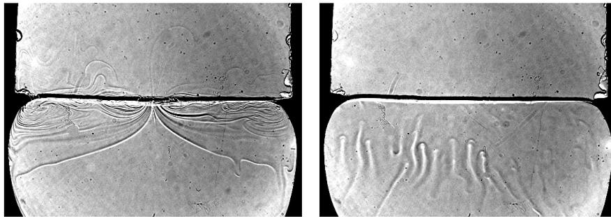
FIG. 1: Marangoni cells (left) and double diffusive fingers (right) which couple during the mass transfer of carboxylic acid undergoing a neutralization in the aqueous phase [1].
