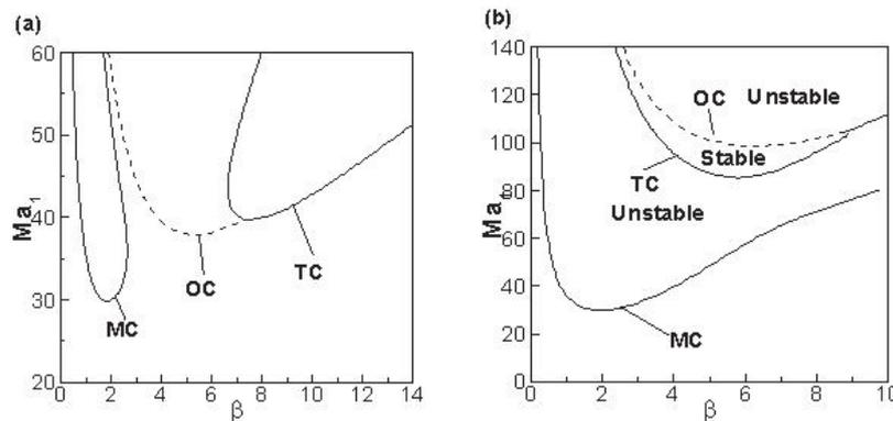
Fig. 1 Marginal curves of the system in  $Ma$ - $k$  plane for Different Biot numbers: (a)  $Bi=30$  and (b)  $Bi=300$ , at same depth ratio  $h$  ( $h_1/h_2$ )=0.5, and streamwise disturbance wavenumber  $\alpha=0$ . The dashed lines correspond to the oscillation mode and the solid lines represent the stationary mode.
