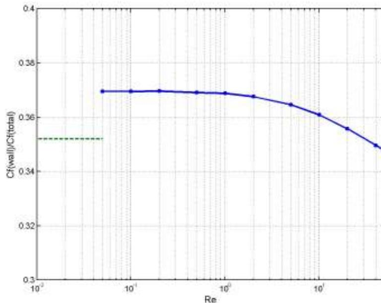
Fig. 1 Variation with the Reynolds number of the relative contribution of the wall shear force.
